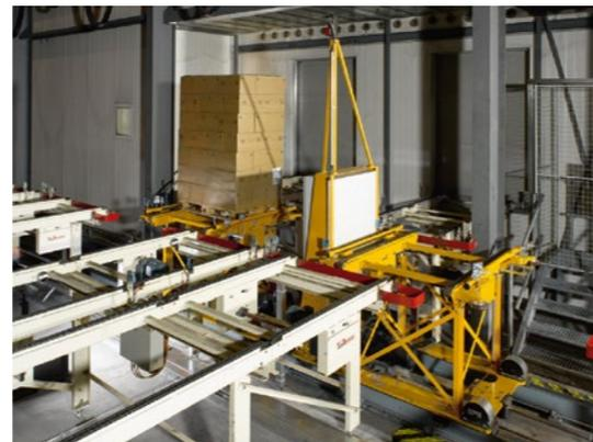
As from 2007, the new and quicker double transfer carriage eliminates a bottleneck in the conveyor technology and, due to a preventive maintenance, runs since then without any problems.
