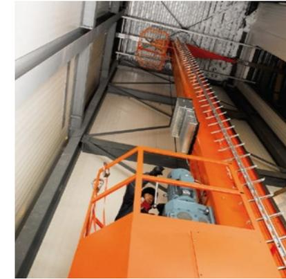
Twelve hours shift at -28° C. The three automated storage and retrieval machines are converted in the service area at the end of the switching aisle.
