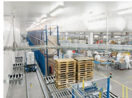
A transfer carriage connects production and packing (on the right) with the high-bay warehouse (on the left) and assists with empty pallet handling.
