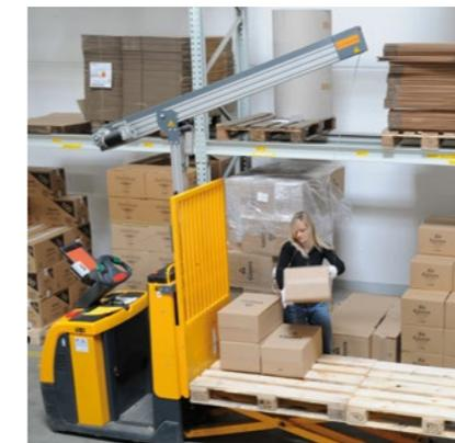
The ergonomic EcoPick® crane takes up to 80% of the strain off the operator during order picking by means of a cable winch and special glove cuffs.
