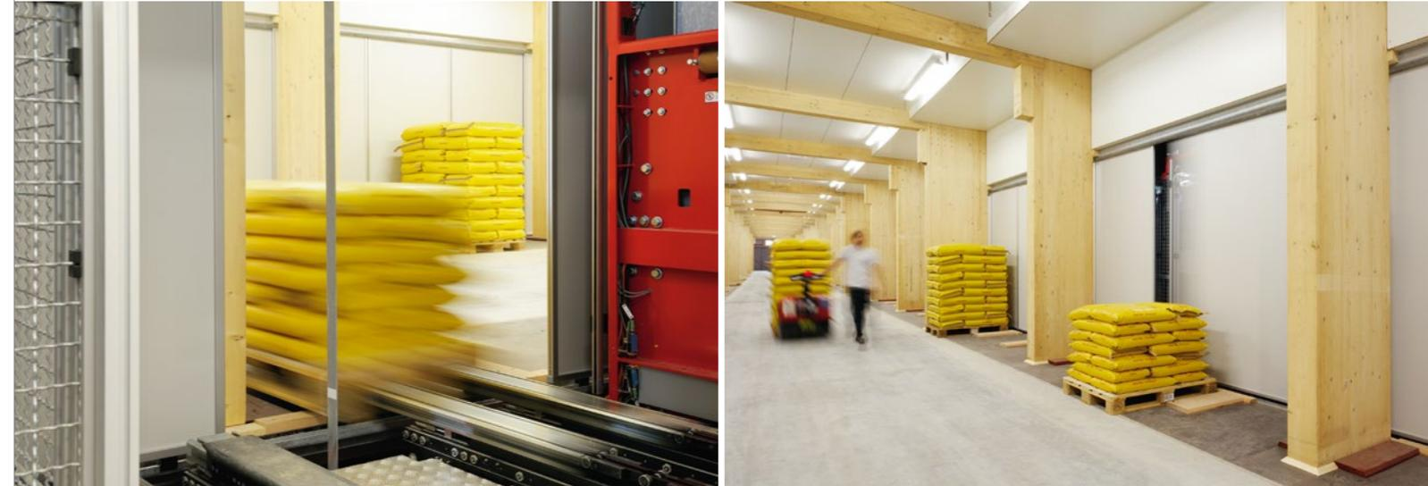
Four stacker cranes supply from both sides three spacious and well-lit order picking tunnels that range over the entire length of the high-bay warehouse. 324 order picking gates by LTW provide safe separation between the tunnel and the stacker crane aisles as required by safety regulations.
