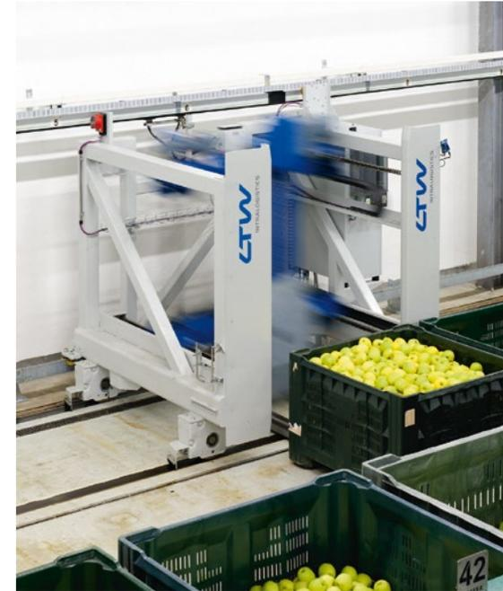
The two-storey, automatic conveyor system between the sorting system and the high-bay warehouse with two transfer cars (picture) and two vertical lifts.
