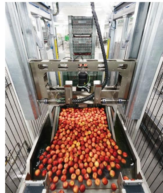
Best evidence for customer satisfaction is a follow-up project: In 2014 LTW installed 16 fully automated fruit dumpers in the pre-zone of the packaging area.
