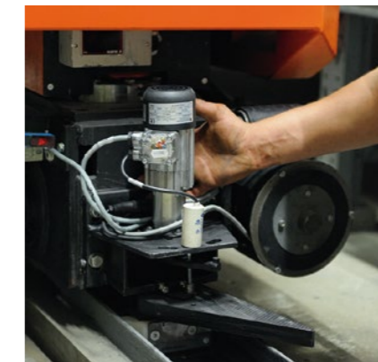
Current (2009) switching technology with redesigned rail-switching drive and rail switches. The new points are built to minimize wear and tear.
