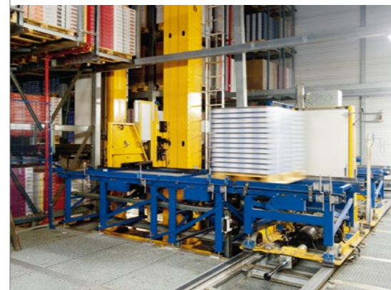
EGGER pallet warehouse with five stacker cranes and complex conveyor system – approved LTW quality in the project phase as well as in long-term usage.
